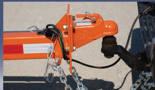
For added versatility, the four-position ball hitch allows the Lo Riser to adjust to various vehicle heights.
