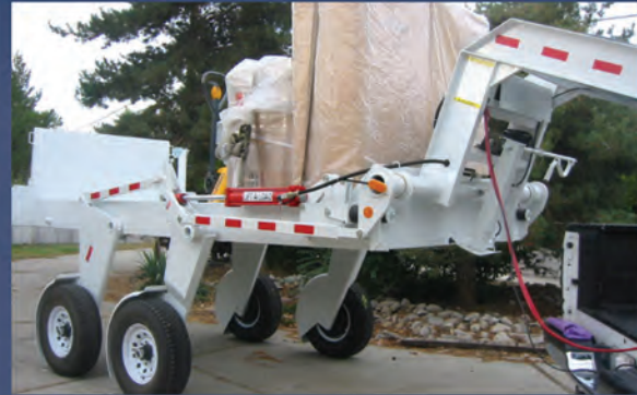
Raised to dock height or truck height, the Lift-a-Load trailers allow for quick loading and unloading.
